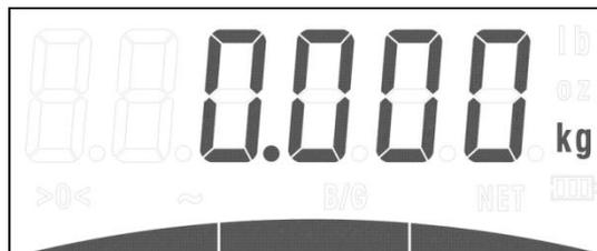
The scale starts to check weighing as soon net weight is greater than 10d.
